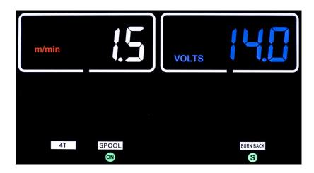
Set wire feed speed using left side knob, adjustable between 1.5 - 15 m/min.
