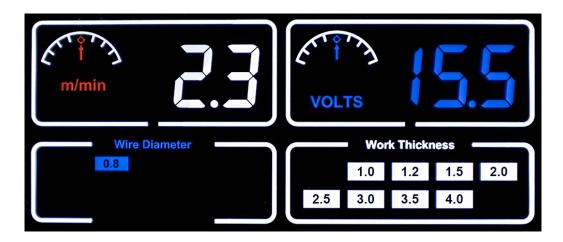
Once you have selected wire size and material thickness the suggested wire speed and voltage will be shown in the display, you are now ready to weld.
