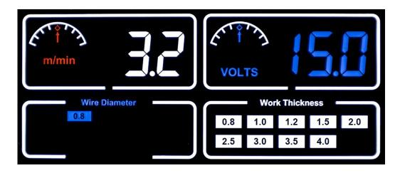
Once you have selected 0.8mm wire size and material thickness the suggested wire speed and voltage will be shown in the display, you are now ready to weld.
