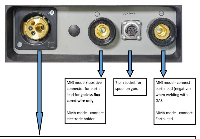
Euro torch connector. Connect Euro type MIG torch to euro torch connector, align torch connector to machine connector and then turn retaining ring clockwise to secure. Ensure torch is secured tightly to avoid weld power problems
